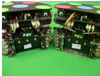
Figure 3. The robot with a straight kicker (left), and the robot with a chip kicker (right).
