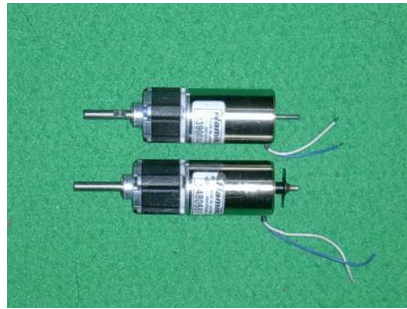
Figure 2. Motor and its modified gearbox.
